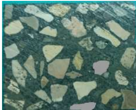
Figure 1. Distribution of coarse aggregates on cross section
