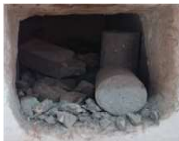
Figure 11. Explosive spalling occurs in cases of SCC and GFSCC mixes in 450 °C
